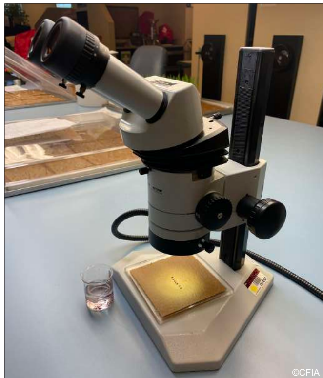
Figure 9.2. Stained seed being examined under a stereo binocular microscope and a beaker of seeds ready for examination as part of the viability (tetrazolium) test (image courtesy of ISTA accredited laboratory CA08)
